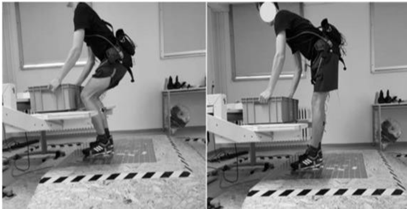
Fig. 4.7. A simulated dynamic lifting task with an exoskeleton using a squatting (left) or prone (right) lifting technique [13]
