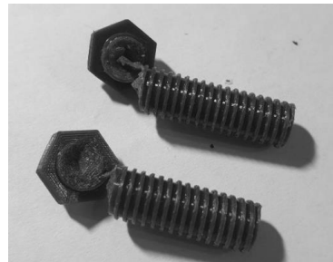
Fig. 6.14. Damaged screws made of PET-G [own elaboration]
