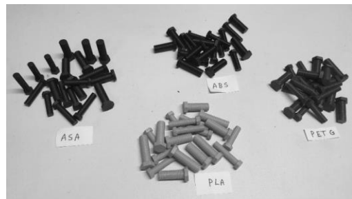
Fig. 6.10. Bolts prepared for testing [own elaboration]
