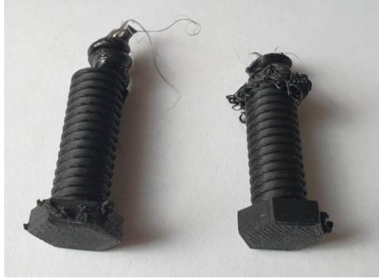
Fig. 6.1. M8 screw made of ASA filament in FDM technology with the selection of incorrect print parameters [own elaboration]
