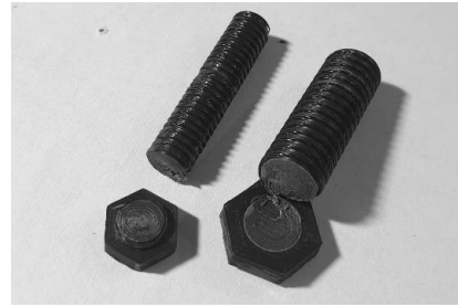
Fig. 6.12. Damaged screws made of ABS [own elaboration]
