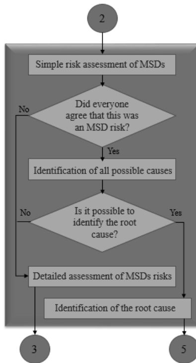
Fig. 2.23. Key steps of implementing Ergonomics prevention programs – implementing MSD risk evaluation [own elaboration]
