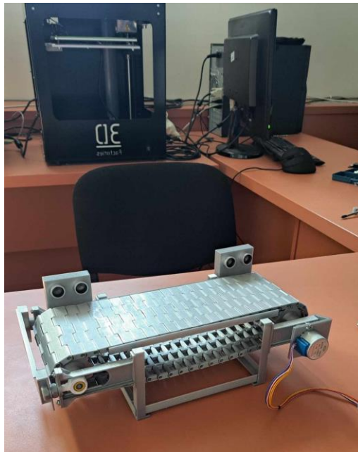
Fig. 4. Printed conveyor belt with ultrasonic device
